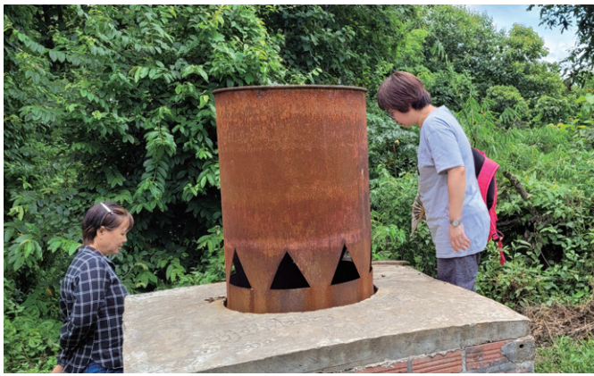
CEDAR staff inspected the small incinerator established in the garbage management project.
